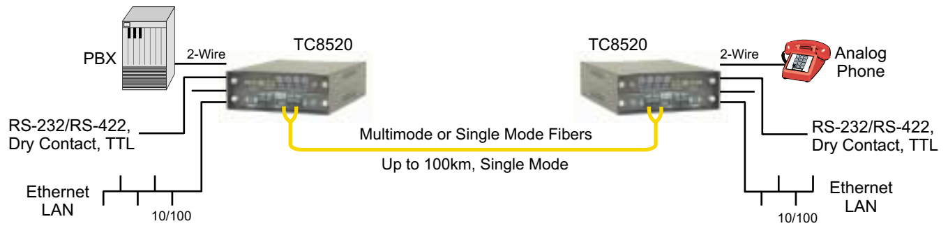
Typical Application Using TC8520 Telephone, 10/100 Ethernet & Serial Data Fiber Optic Multiplexers.
